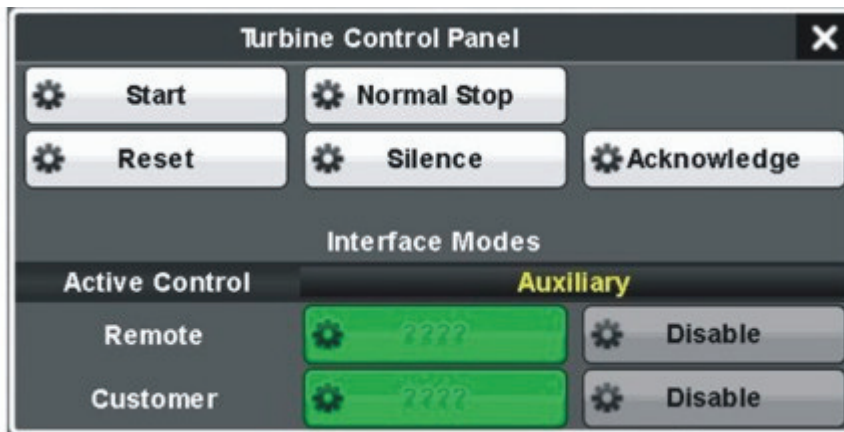
Figure 4.2.1 Turbine Control Panel (TCP) Window
