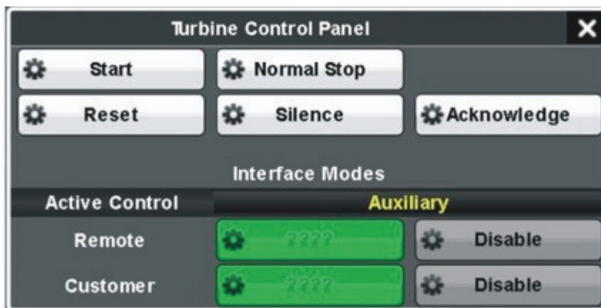
Figure 4.3.1 Turbine Control Panel (TCP) Window
