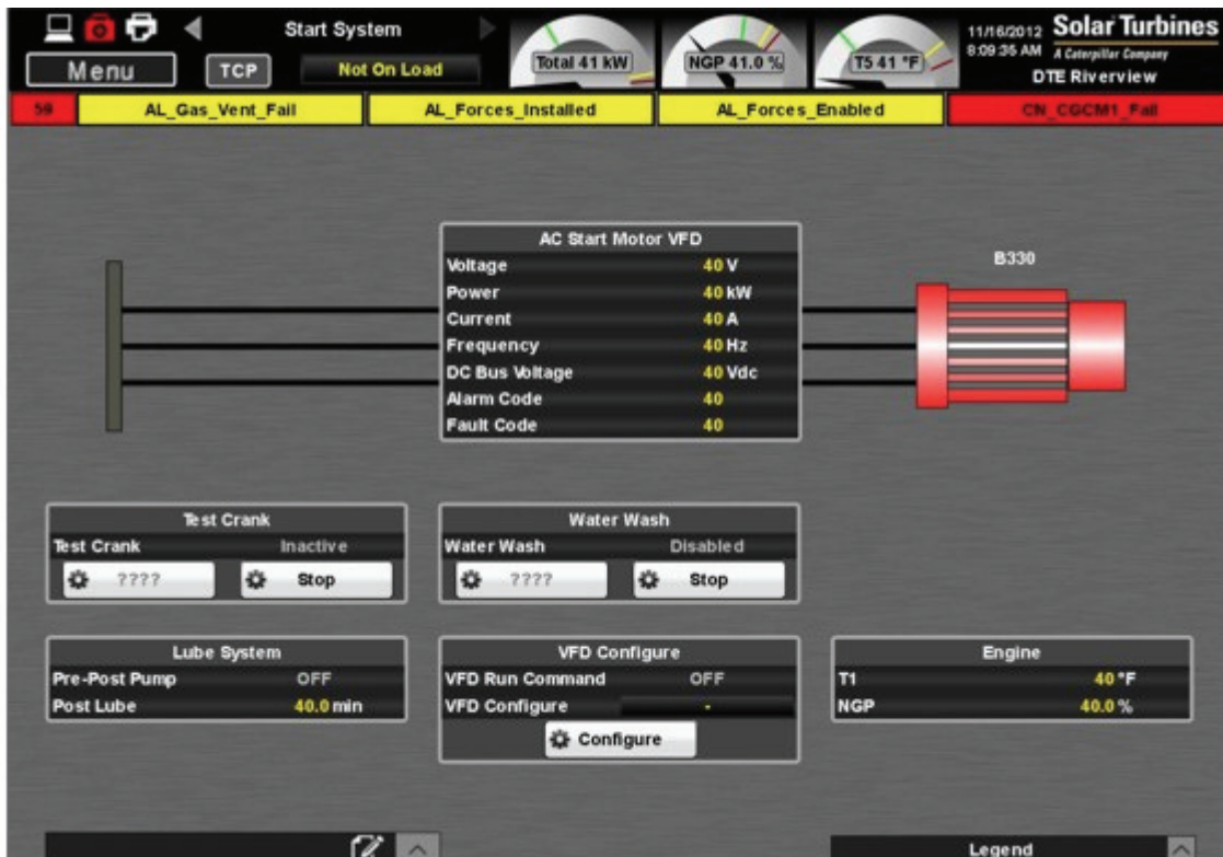
Figure 3.3.8 Start System Screen
