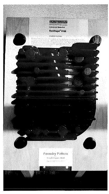
Image 3(Small Eng Block Mold): Small Engine Block mold
