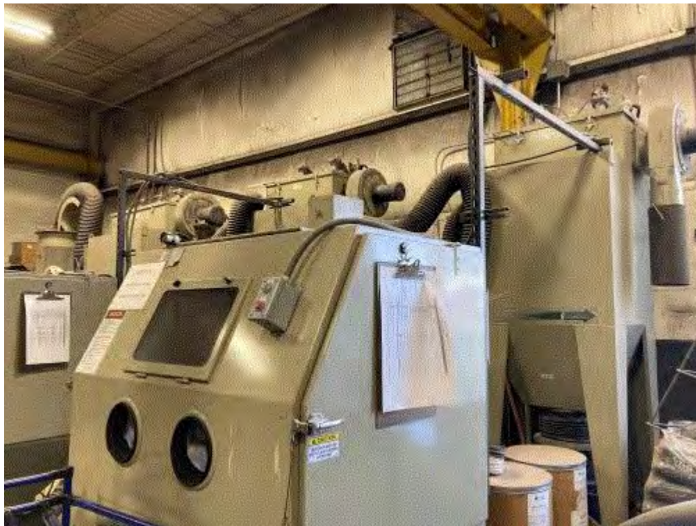
Image 6(Shot Blasting) : Aluminum Oxide shot blasting stations, vented to in-plant environment
