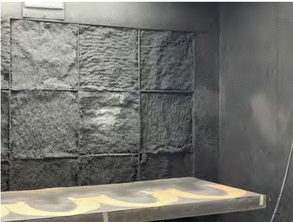
Image 4(Coating Booth 2) : Coating booth filters with gaps and buckles around edges.
