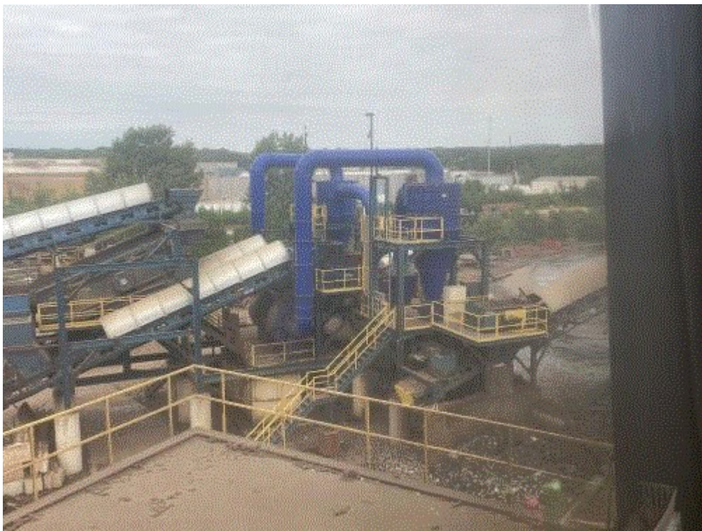
Image 10(Non ferrous system) : New non ferrous separation system, from shredder operator tower view.
