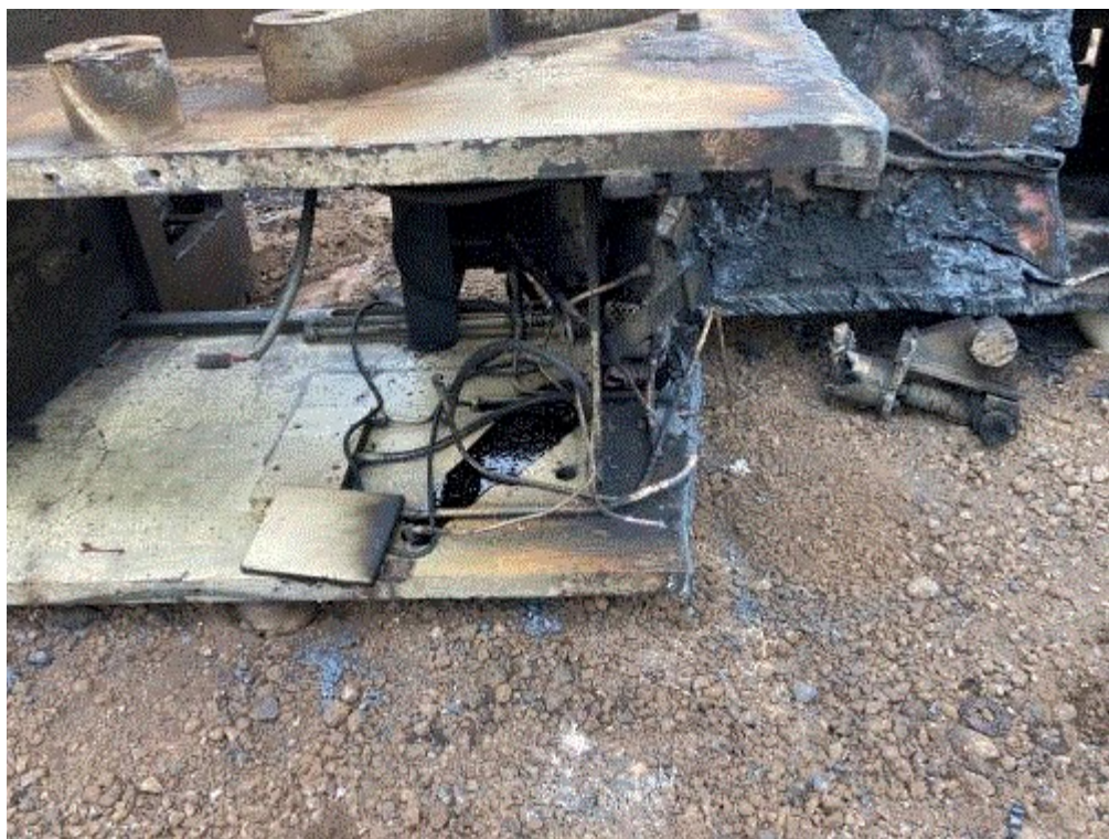
Image 2(Torched press) : Oil leaking from press being torched. 8/23/23
