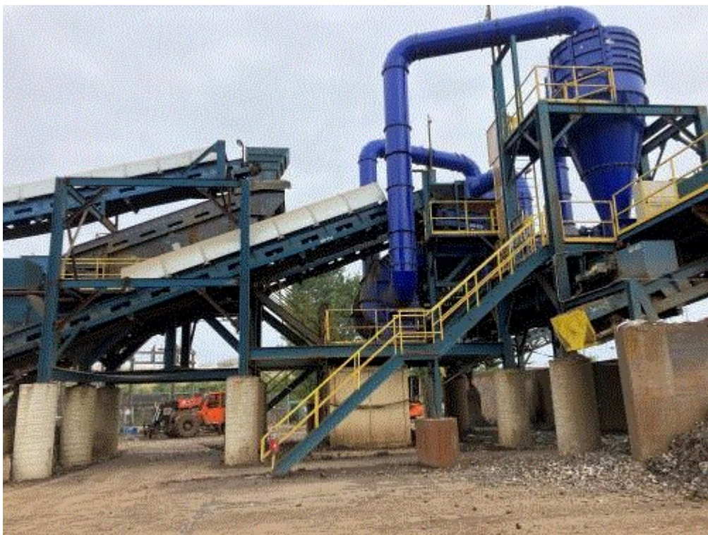
Image 5(New emission unit) : New non-ferrous material separation system. 8/23/23
