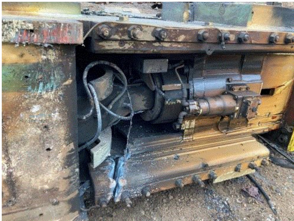
Image 3(Torched hoses) : Hoses being torched on press. 8/23/23
