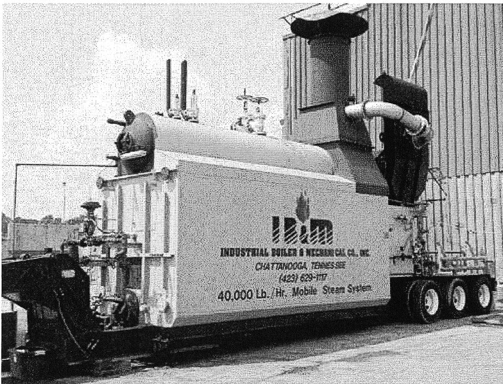
**Image 1(20150701 114501 v2) :** EUTEMPBOILER conical rain cap on exhaust stack. Per permit engineer, dispersion modeling of air toxics was independent of exhaust stack parameters. Therefore, this noncompliance with PTI 180-14, VIII is insignificant. Cap has been removed by source.
