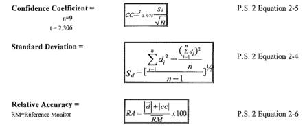
RA calculated as specified in Performance Specification 2, Appendix B, 40 CFR 60 - Equation 2-4
