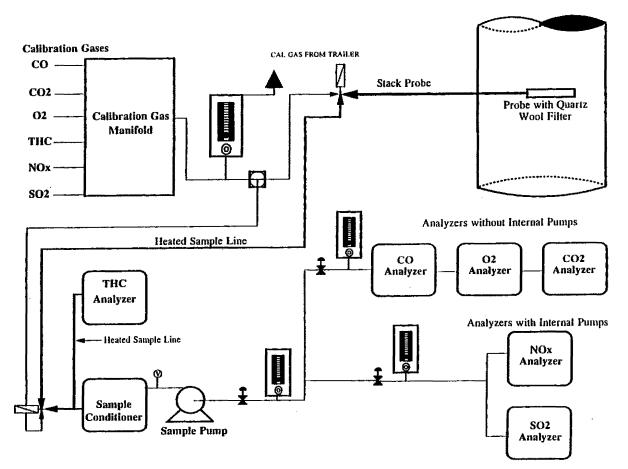
**Figure 3-1. CEM Sample Flow and Calibration System** Note: This study used the CO<sub>2</sub> and O<sub>2</sub> analyzers.
