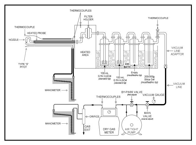
FIGURE 3-1 US EPA METHOD 26A (HALIDES) SAMPLING TRAIN
