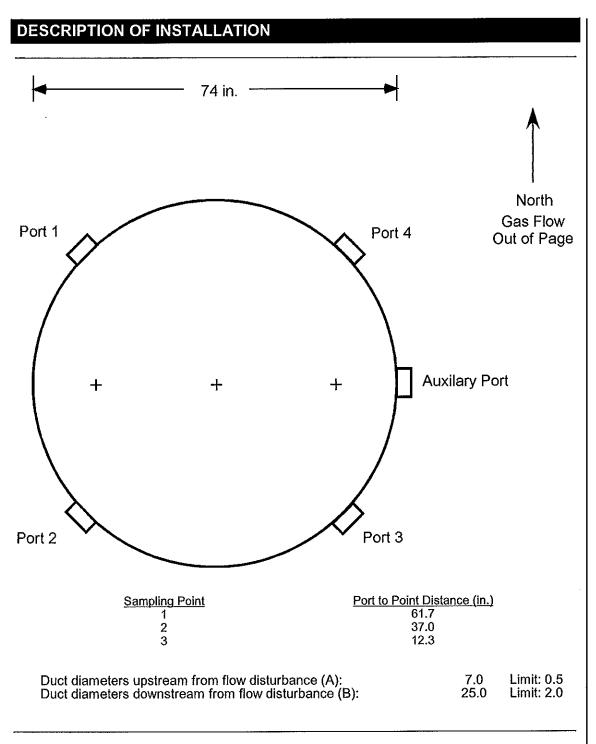
Figure 3-1: USEPA Method 3A/7E Sampling Points – RATA and Emissions Testing
