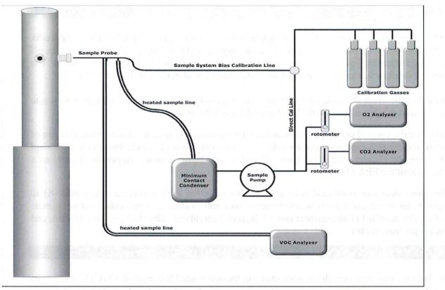
Figure 1: Example Erthwrks Gaseous Sampling System Diagram
