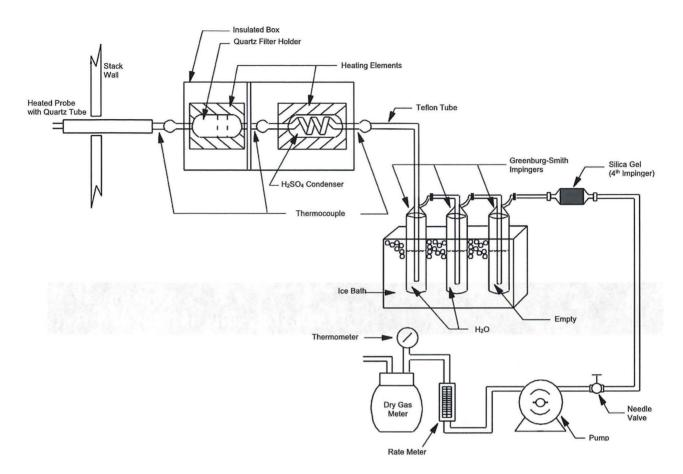
Figure 2: Example Erthwrks CTM-013 Sample System Diagram
