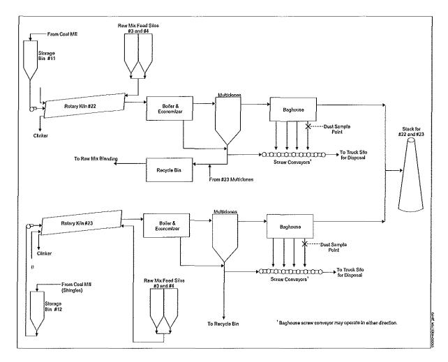
Figure 3-1. Process Flow Diagram for Kiln Group 6
