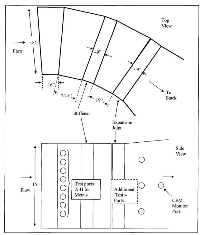
Figure 3-2. Kiln 23 Breeching Ducts
