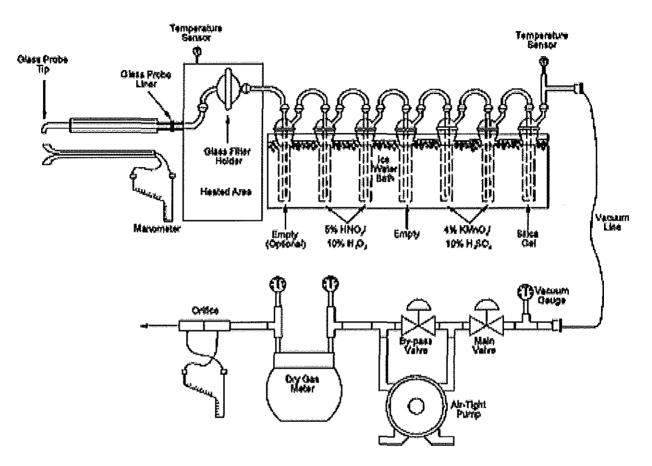
Figure 4-1. Method 29 – Multi-Metals Train Schematic
