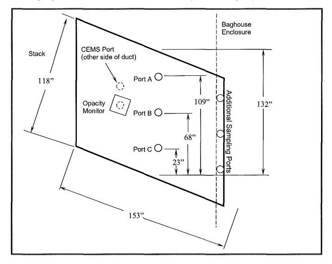
Figure 4-1. Kiln 19 Test Port Locations (side view)
