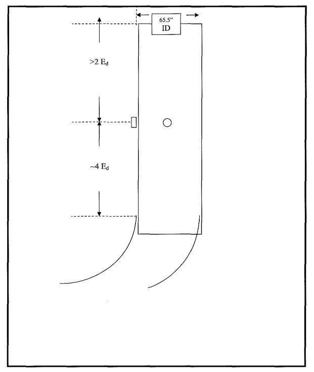
Figure 4-5. Raw Mill Stack Locations
