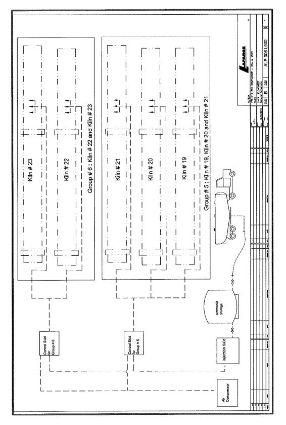
Figure 3-2. Schematic of Kiln Group 5 and Kiln Group 6 SNCR System
