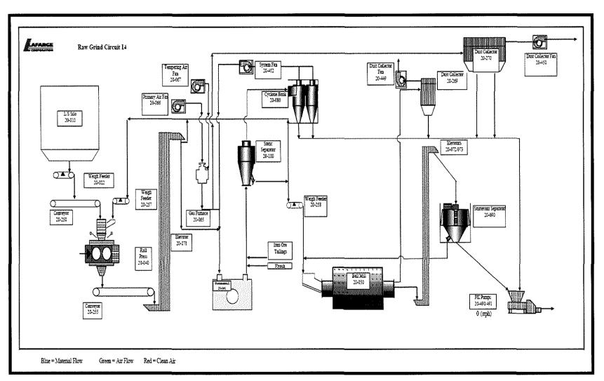
Figure 3-3. Raw Mill Process Diagram
