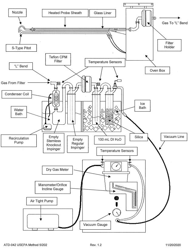
USEPA Method 5/202- Filterable/Condensable Particulate Matter
