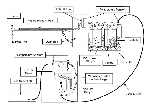
USEPA Method 5- Particulate Matter Sample Train Diagram
