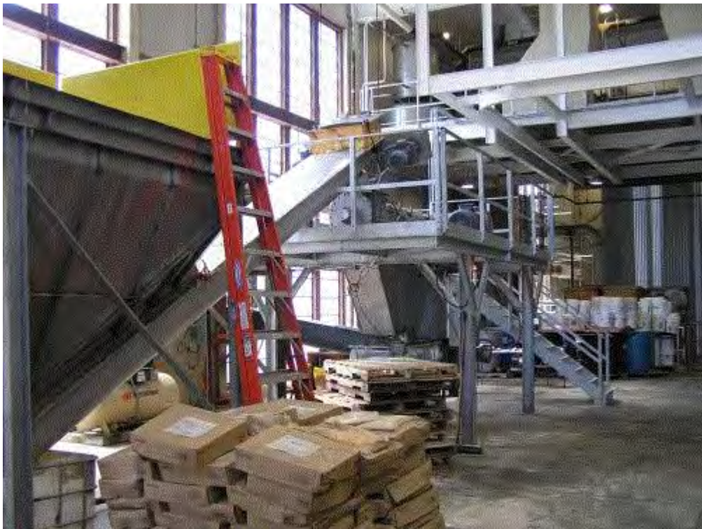
Image 7(007) : Hopper at left, and depackager at center of photo.
