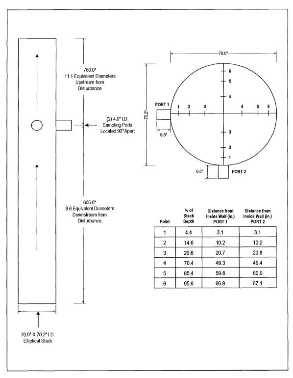
FIGURE 2-1 BOILER NO. 8 EXHAUST TRAVERSE POINT LOCATION DRAWING
