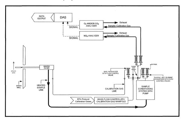
3.1.5 EPA Method 19, Determination of Sulfur Dioxide Removal
