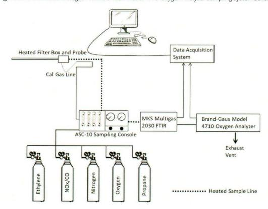
The ASC-10ST was used to deliver calibration gases (Calibration Transfer Standard (CTS), QA Spike and Nitrogen) to the FTIR in direct (to analyzer) and system (to probe) modes.
