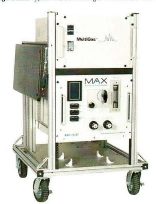
Figure 5.2b: Typical MKS 2030 Multigas FTIR and ASC-10ST Configuration
