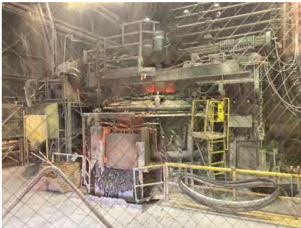
Image 14(EAF) : EAF half way through melt cycle.
