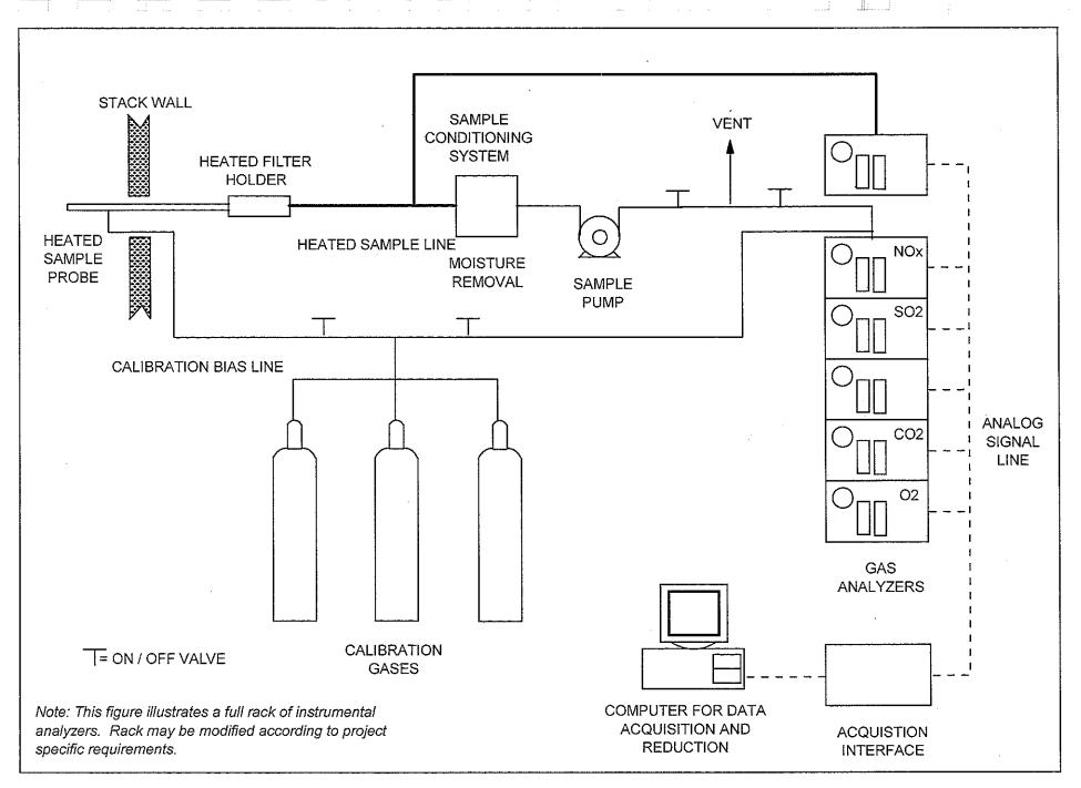
FIGURE 4 - 1 WESTON SAMPLING SYSTEM Interference checks were performed prior to mobilization as per the applicable reference method. The NOx analyzer NO<sub>2</sub> to NO converter efficiency was performed prior to and after the test effort in accordance with EPA Reference Method 7E.
