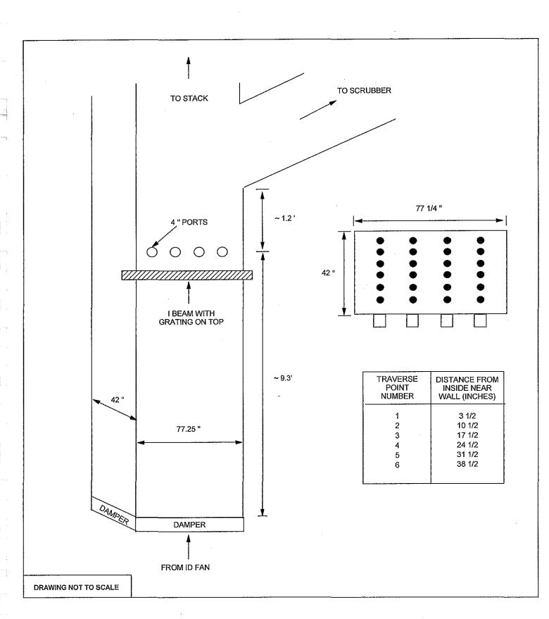
FIGURE 3-1 WPEP BOILER NO. 1 - LOWER DUCT TEST PORT AND TRAVERSE POINT LOCATIONS
