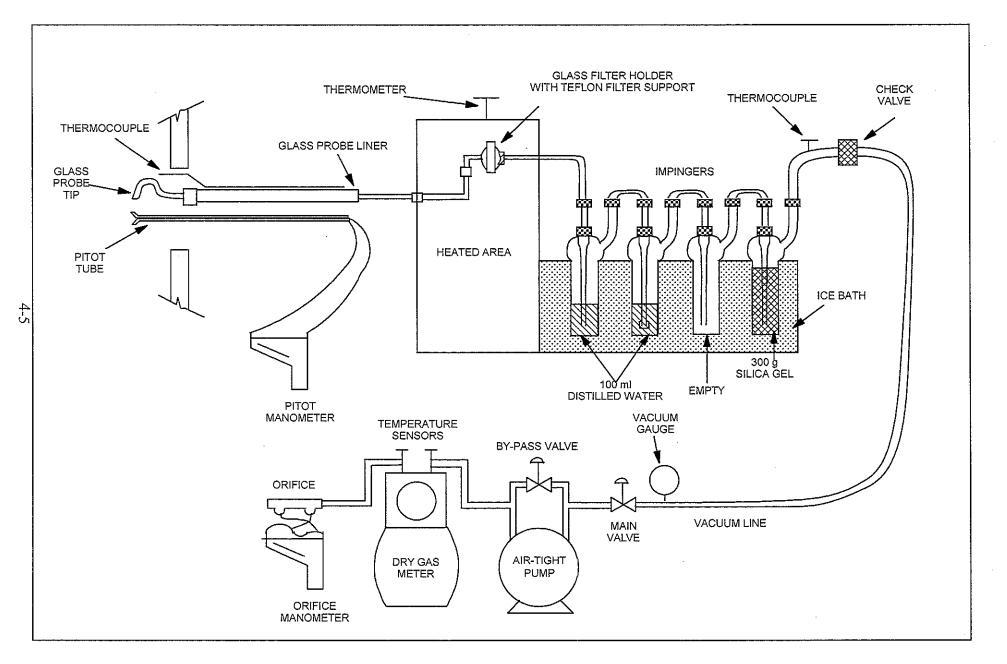
FIGURE 4-2 EPA METHOD 5 PARTICULATE MATTER SAMPLING TRAIN
