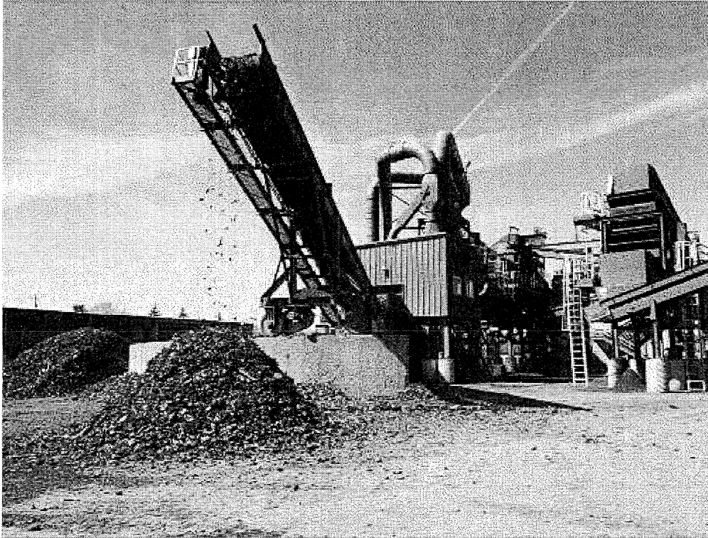
Image 3(Metal shredder) : Metal shredder, z-box, cyclones and other associated equipment.
