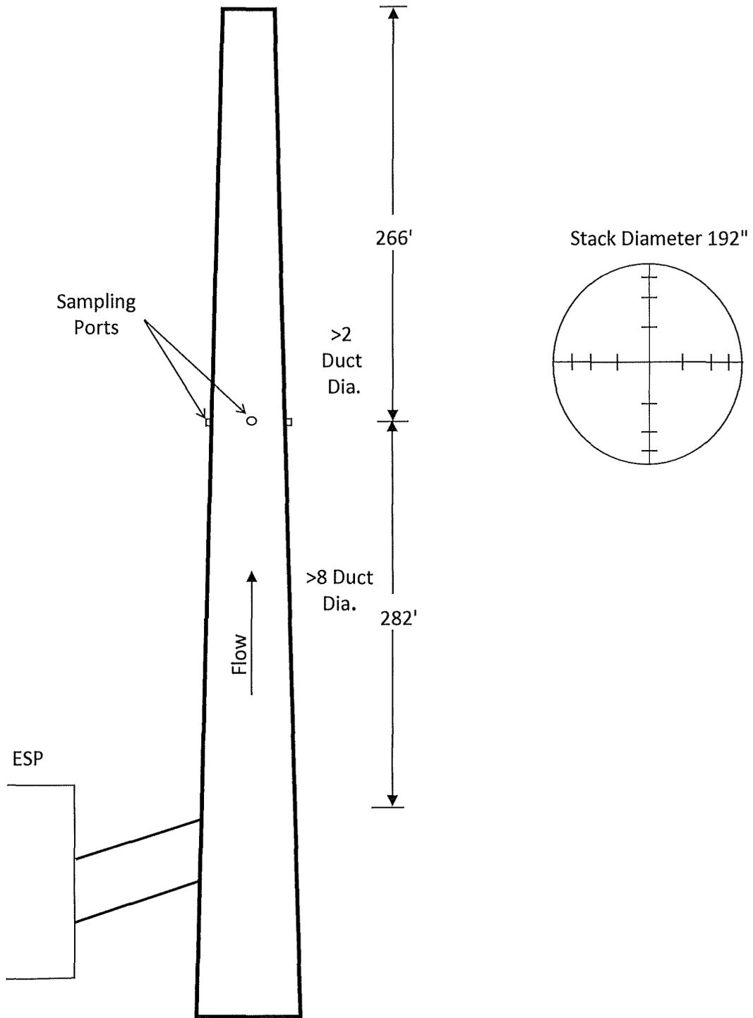
Figure 2 – USEPA Method 26A (Modified)
