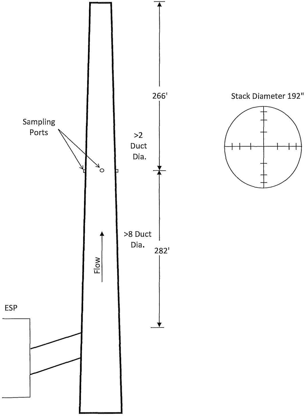
Figure 2 – USEPA Method 26A (Modified)
