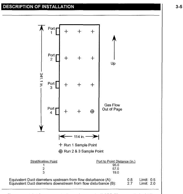
Figure 3-3: Unit 2 Sampling Point Determination - 100% PRB (Mod. EPA Method 3A)
