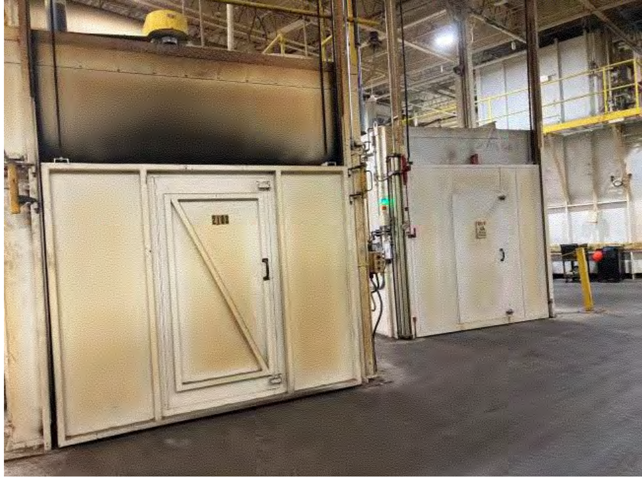
Image 3(Heat Treating ovens) : Used to heat treat aluminum
