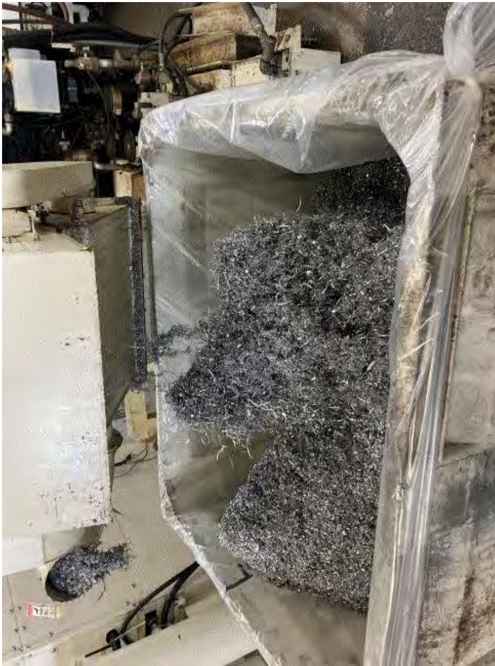
Image 1(Aluminum Shavings) : These are the aluminum scrap that are not reused, but sent to a 3rd party to readjust the material's chemistry.
