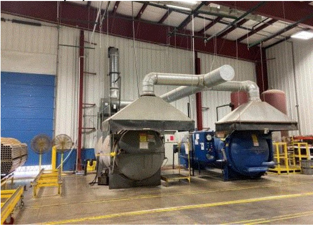
Image 1(Electric Autoclaves) : 2 old autoclaves with a hoods that go to a combined stack with raincape.
