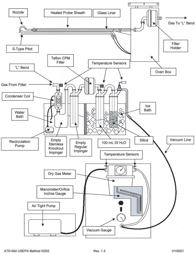
USEPA Method 5/202- Filterable/Condensable Particulate Matter
