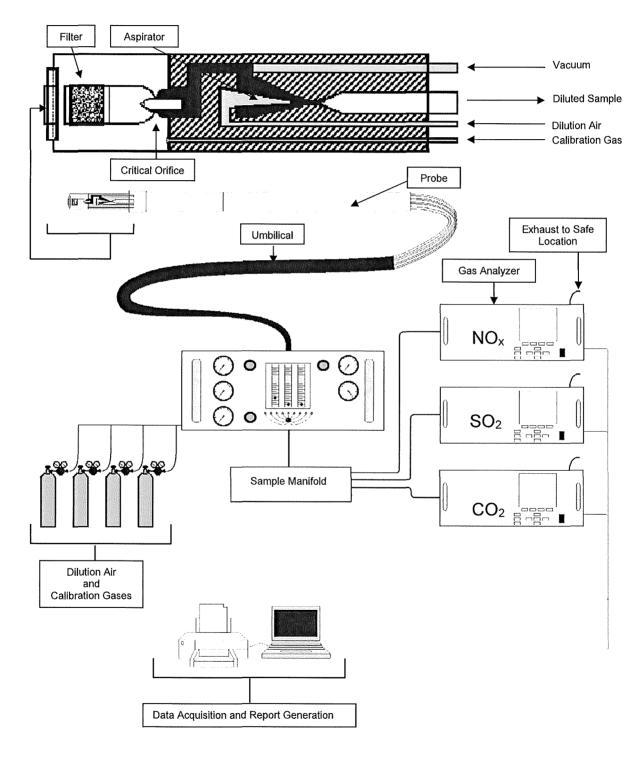
ATD-018 In-Stack Gas Dilution 3A 6C and 7E
