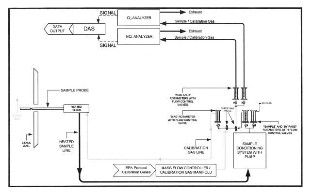
FIGURE 3-1 EPA METHODS 3A (O<sub>2</sub>), 7E SAMPLING TRAIN
