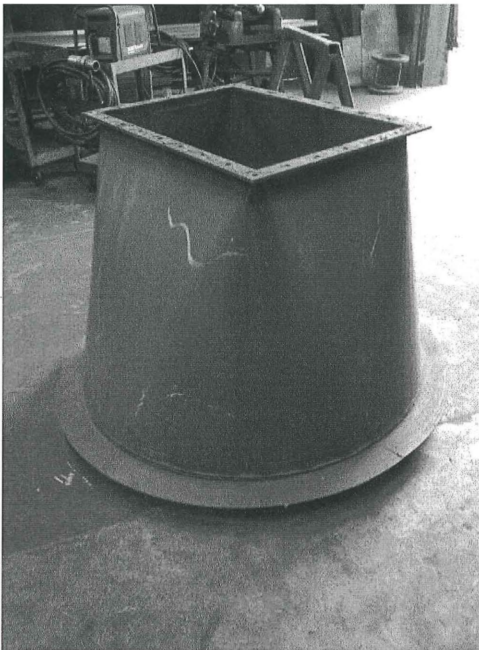
Image 2(LWEC new hood) : Replacement hood for cyclone fuel receiving hopper. Photo taken on 8/27/2015.
