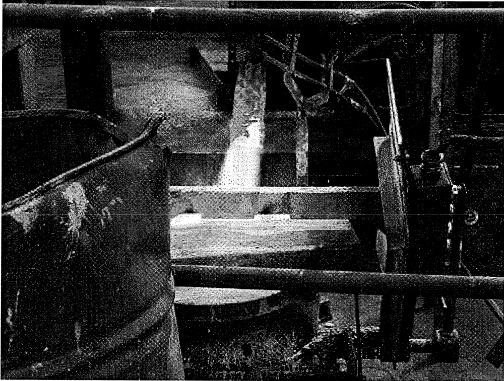
Image 6(Natural gas torch) : Natural gas torch heating ladle
