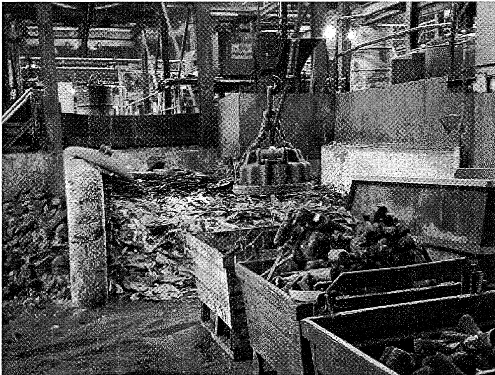
Image 3(Scrap metal storage) : Scrap metal that is being lifted by a magnet to be carried to melt furnaces.
