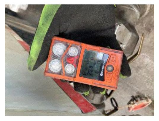
Image 4(LEL Meter) : Meter used to check for leaks. Reading was "0" during inspection.
