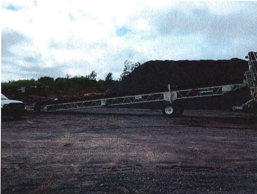
Image 2(SSG1) : T-320 Conveyor
