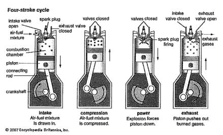
Figure 3-1 Four-Stroke Engine Process Diagram
