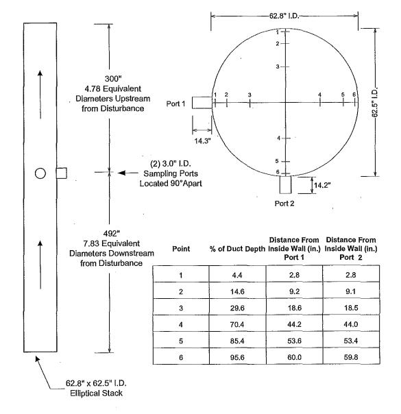
Figure 3.2 - BRF SVREHEAT-FRN Exhaust Stack Traverse Point Location Drawing
