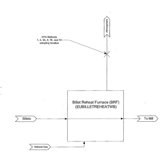
**Figure 3.1 - BRF Process and Sampling Location Schematic**
