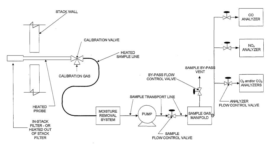
Figure 4.2 - EPA Method 3A, 7E, and 10 Sampling Train Schematic
