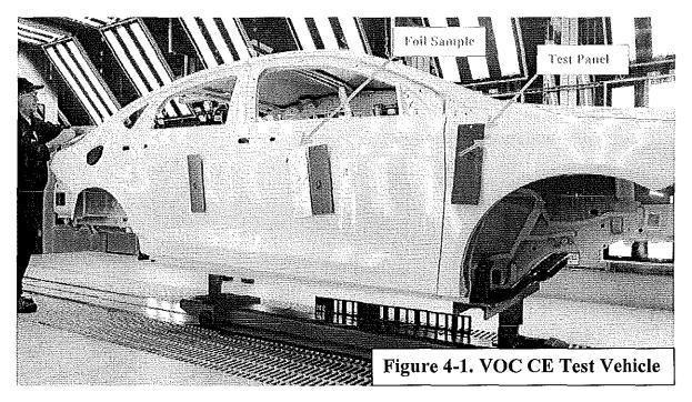
The VOC CE was measured by routing one test vehicle through the coating line with clean, labeled, pre-weighed electrocoated coated and baked 4-inch-by-12-inch panels attached to the exterior body and interior of the vehicle using magnets. The panels were positioned at locations where:
