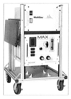
Figure 4.2.1: Typical MKS MultiGas 2030 FTIR and ASC-10ST measurement system
