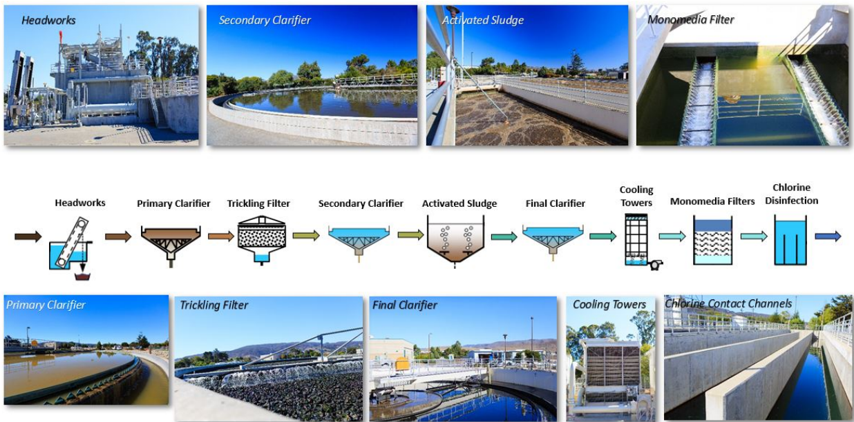
FIGURE 13 SIMPLIFIED OVERVIEW OF THE WRRF OPERATIONS
