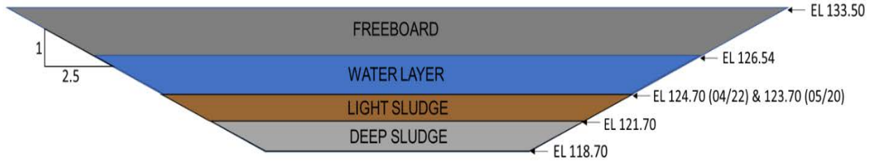
FIGURE 15 ELEVATION DRAWING OF THE EXISTING LAGOON SYSTEM
