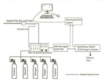
The ASC-10ST was used to deliver calibration gases (Calibration Transfer Standard (CTS), QA Spike and Nitrogen) to the FTIR in direct (to analyzer) and system (to probe) modes.
