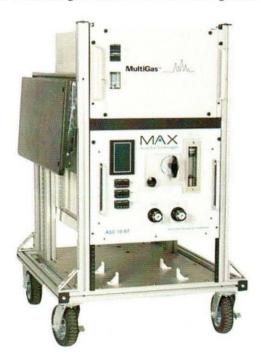
Figure 5.2b: Typical MKS 2030 Multigas FTIR and ASC-10ST Configuration
