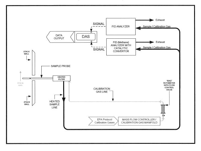
FIGURE 4-4 EPA METHOD 25A (TGO AND METHANE) SAMPLING TRAIN
