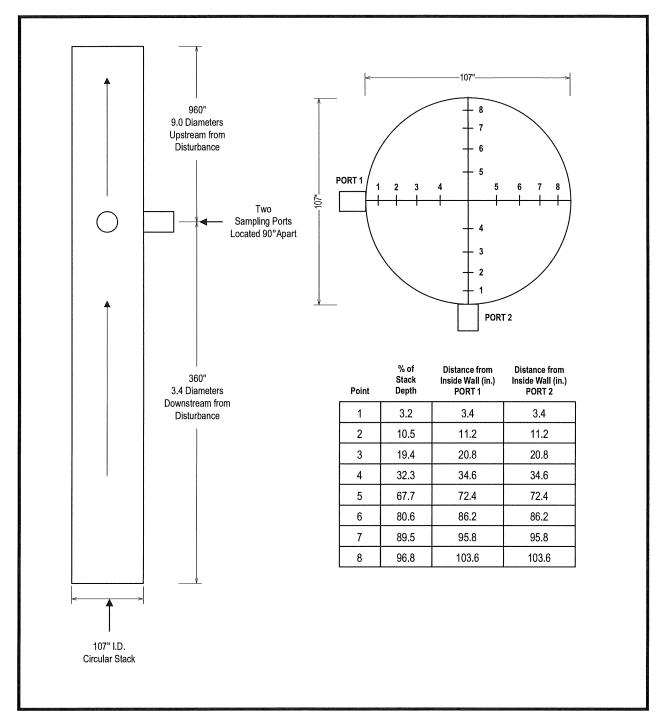
FIGURE 4-7 RCO B OUTLET EXHAUST FLOW TRAVERSE
