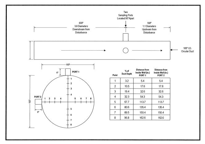
FIGURE 4-5 RCO A, B, AND C COMBINED INLET FLOW TRAVERSE
