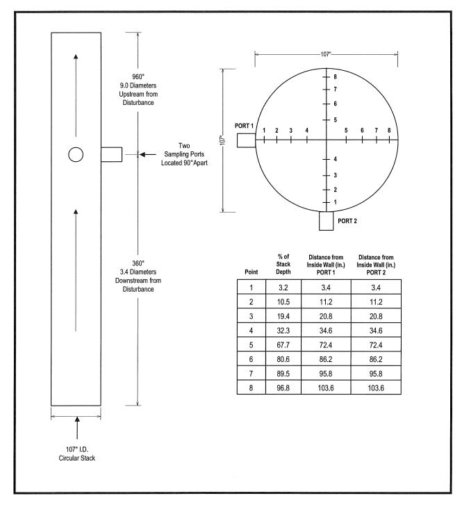
FIGURE 4-6 RCO A OUTLET EXHAUST FLOW TRAVERSE
