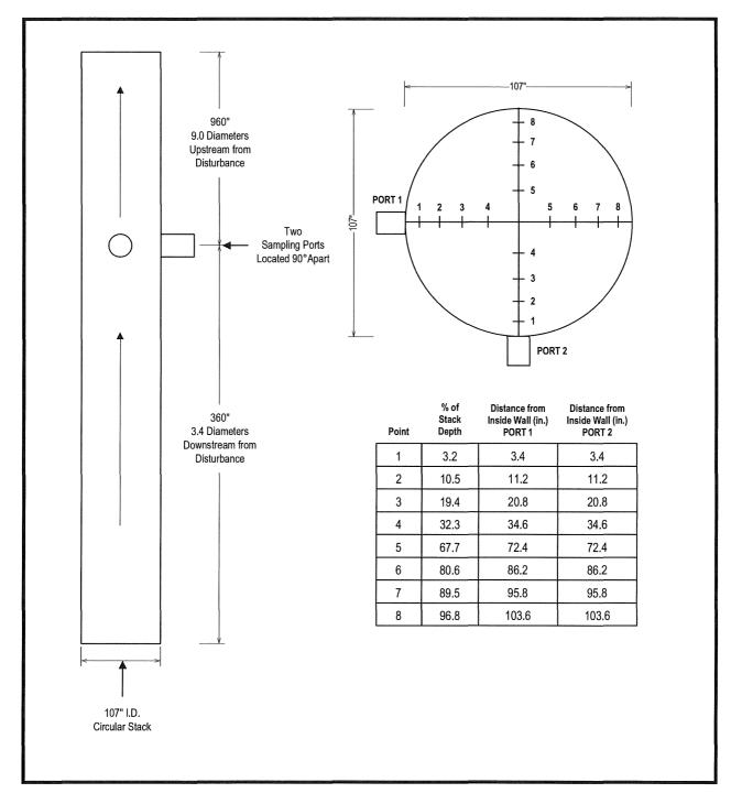
FIGURE 4-8 RCO C OUTLET EXHAUST FLOW TRAVERSE
