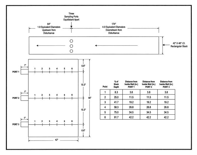
FIGURE 4-10 RTO OUTLET EXHAUST FLOW TRAVERSE
