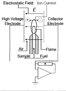
Figure 4-3. FID Flame Chamber
