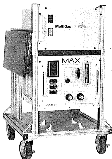
Figure 3: Typical MKS MultiGas 2030 FTIR and ASC-10ST measurement system
