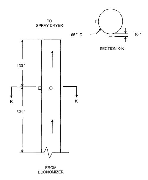
Figure 4-1. SDA Inlet Sampling Location (Units 1 & 2 are identical)
