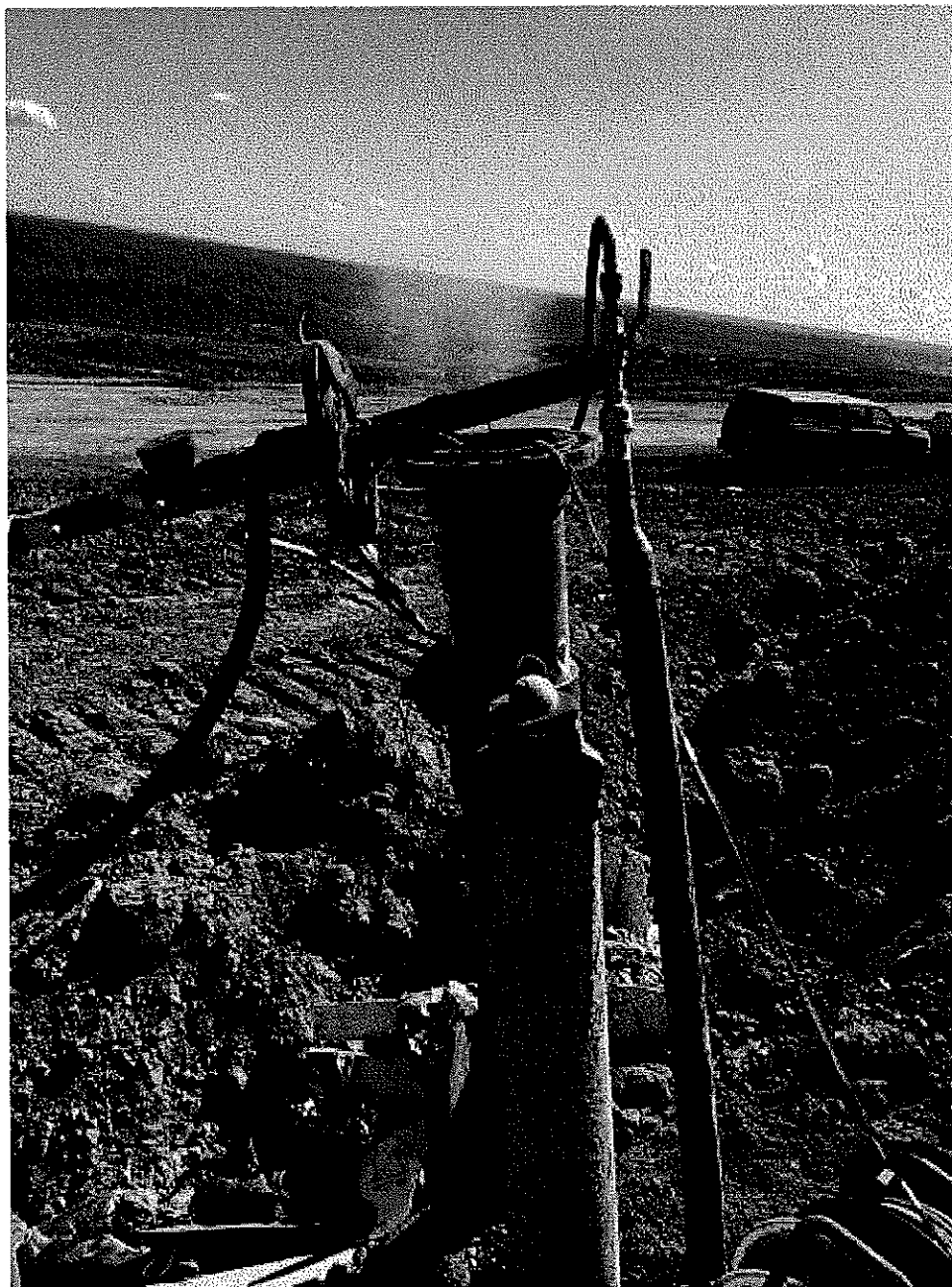
Image 1(Top removed-well) : Top removed from well head to do downhole temperature test.
