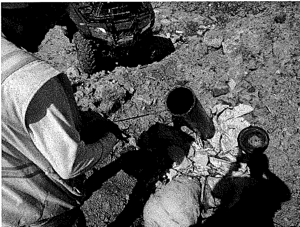
Image 7(Down hole test) : Down hole temperature testing.
