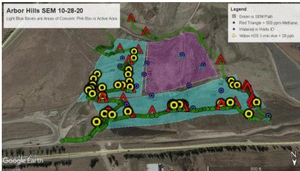
Image 1(SEM Path) : SEM Path along with SEM methane hits and areas where H2S was above 20 ppb.(Yellow circles.)
