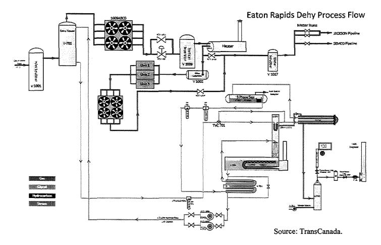
Figure 2-2. Eaton Rapids Dehydration Unit Process Flow
