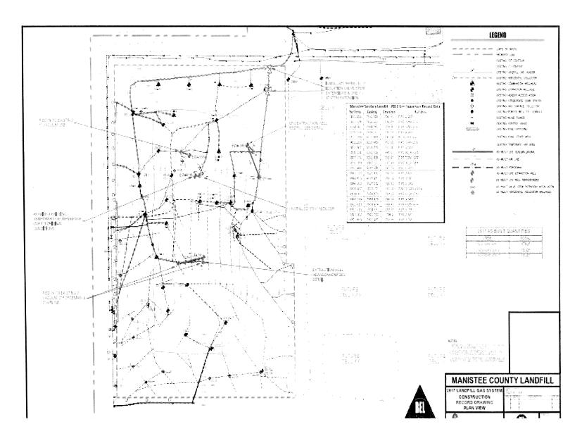
Figure 1: Manistee County Landfill Gas Collection System - General Arrangement
