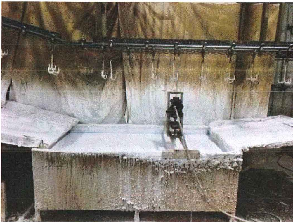
Image 3(Dip Container) : A surface coating line for fence posts containing an open dip tank of low-VOC paint.
