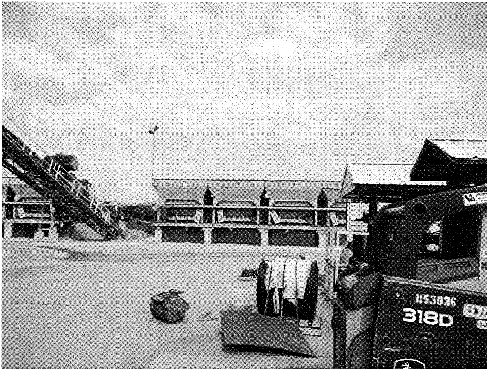
Image 2(Figure 2) : The cold feed aggregate bins, 8/28/15, 10:15 am.
