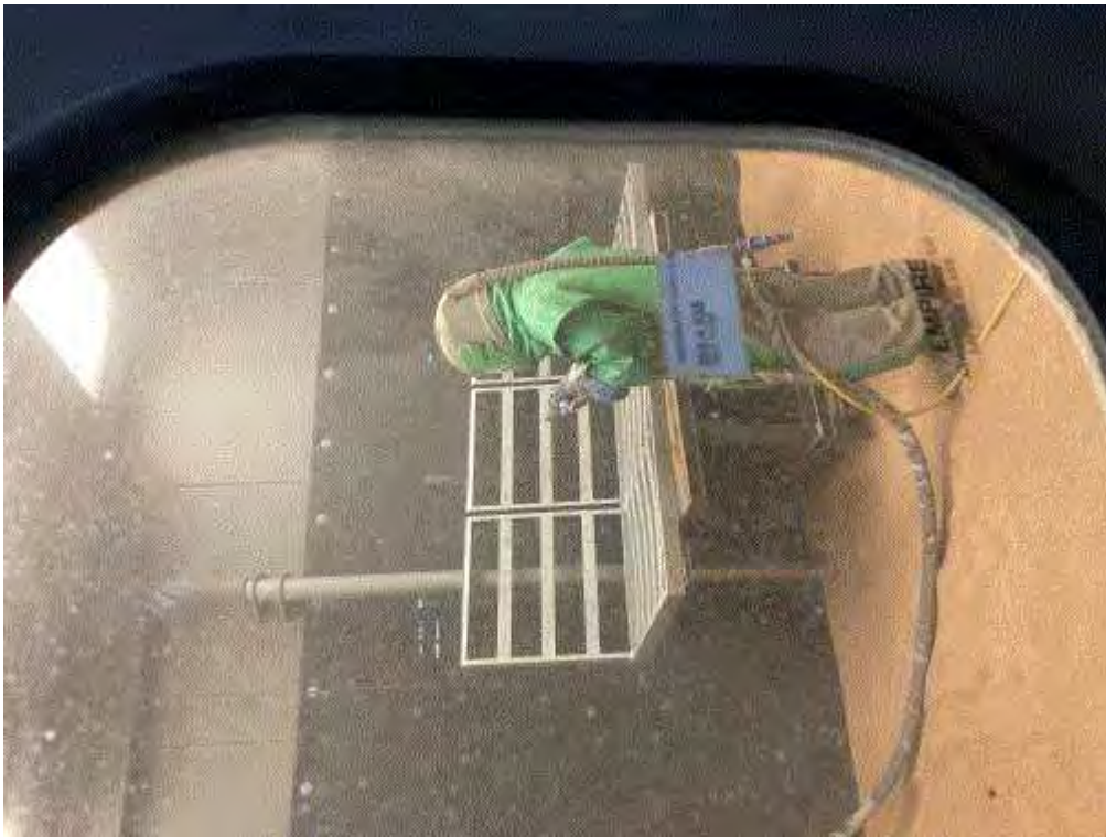
Image 4(IMG_0130) : Aluminum parts cleaning booth
