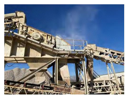
Image 3(Fugitive Dust 3): 5 x 12 Screen (S1) and fugitive dust in excess of 10% standard.
