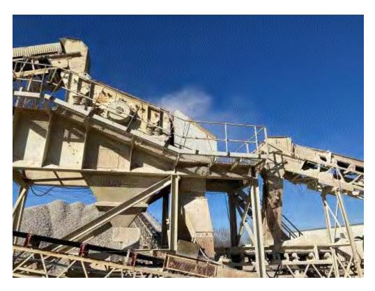
**Image 1(Fugitive Dust 1):** 5 x 12 Screen (S1) and fugitive dust in excess of 10% standard.
