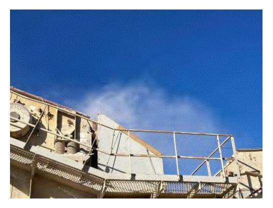
Image 2(Fugitive Dust 2): 5 x 12 Screen (S1) and fugitive dust in excess of 10% standard.
